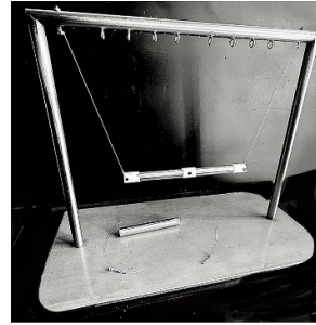
Figure 2. Experimental setup of the doubly suspended pendulum: the long bar has markers attached at its endpoints and at its centre of mass.
