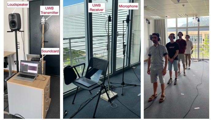
Fig. 3. Transmitter (left) and receiver (middle) apparatus; NLOS setup (right).
