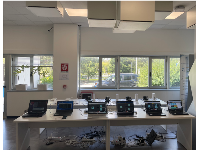
Fig. 3. A picture of the setup of the 5G SA architecture, showing the base station, the six CPEs, the four NMP devices, the four headphones, the sound card, the six laptops, and the smartphone.
