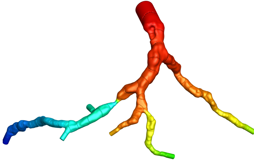
Figure 1.18: Coronary tree test. Pressure distribution among the entire domain.
