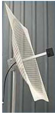
Fig.6. Parabolic directional antenna installed at the remote site
