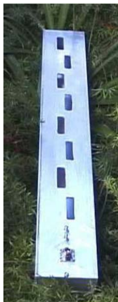
Fig.5. Slotted waveguide (omni-directional) antenna employed at the gateway
