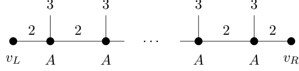
Figure 6.25: Example of a homogeneous matrix product states with open boundary conditions with bond dimensions equal to 2 and local dimensions equal to 3. Each inner vertex is associated with the same tensor A \in (\mathbb{C}^{2 \times 2})^{\times 3} , with A_i \in \mathbb{C}^2 for every i = 1, 2, 3 . The boundaries are vectors v_L, v_R \in \mathbb{C}^2 .
