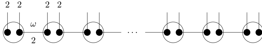
Figure 5.9: On each site, we consider a pair of spin 1/2. Every nearby pair of spin 1/2 in different sites are put in a spin singlet . The pair of spin 1/2 inside each site can have only spin either 0 or 1.
