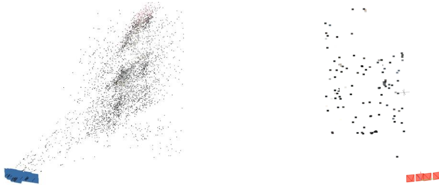
Figure 4-19. Incorrect image orientation in Metashape and COLMAP.
