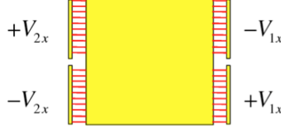
Figure 2.3: Actuation configuration for the x degree of freedom with actuation scheme of constant stiffness and TM voltage zero. The amplitude voltages applied on the four electrodes are indicated in the figure.
