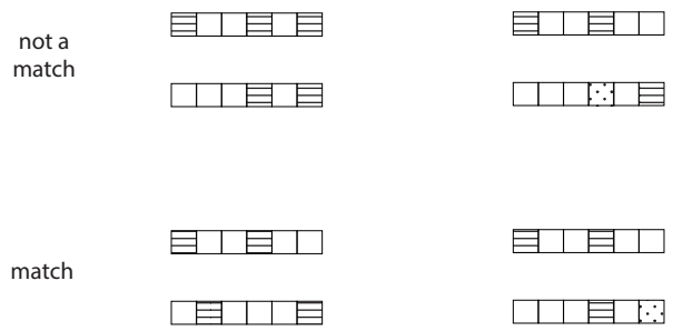
Figure 5.12: Sentominos are defined to match if they have no overlapping valorized position or if they contain matching values in all their common valorized positions (bottom part of the picture). On the other hand, they do not match if one is a subset of the other or if their common valorized positions do not match.
