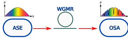
FIGURE 2.5: Schematic representation of the experimental setup for the broadband characterization of the photonic structures, in the NIR wavelength range. An ASE source emits broadband, incoherent and unpolarized, light, in the range from 1530 to 1570 nm. The light is transmitted through the WGM resonator sensor and analyzed at the output with an OSA. The transmission spectrum is retrieved in a single acquisition.
