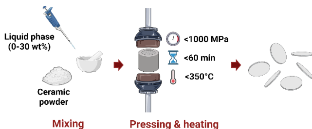
Figure 7 Cold sintering process scheme.
