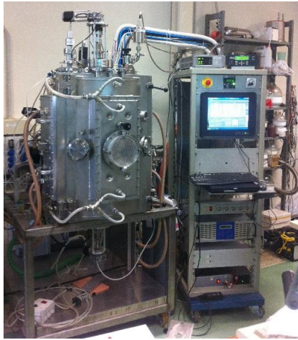
Figure III-18. Prototype of PVD reactive magnetron sputtering system.
