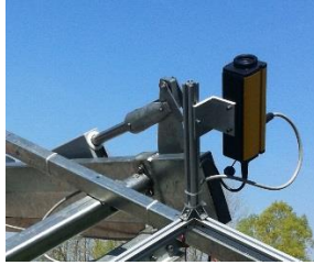
Figure III-37. AKKUtrack™ solar tracking systems.
