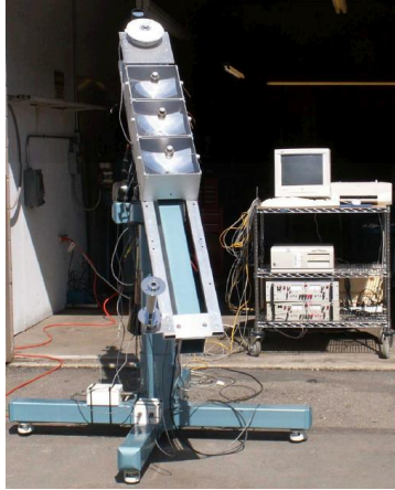
Figure II-10. Cassegrain CPV modules on 2-axis solar tracker.
