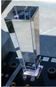
Figure III-12. Optical glue material between sun-rod and CPV cell.
