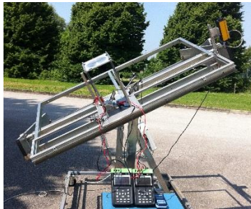
Figure IV-79. CPV prototype spectra spitting system.
