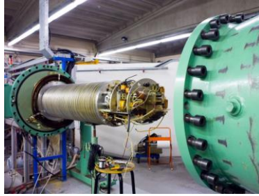
Figure III-24. Van de Graaf AN2000 accelerator at LNL-INFN Legnaro-Padua.
