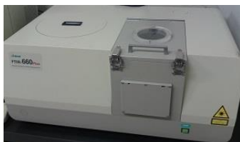
Figure III-23. FT-IR spectrometer Jasco FT-IR 660 Plus.
