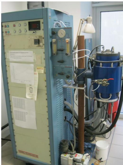
Figure 2-6: Astro high temperature graphite furnace
