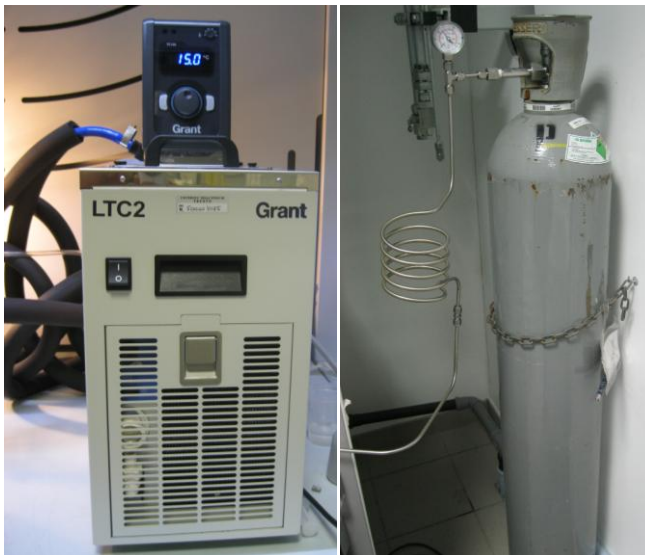
Figure 2-4 : Thermostated water bath and liquid CO 2 tank
