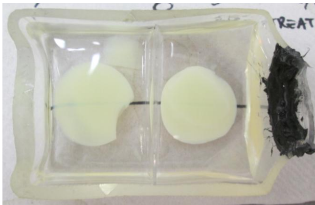
Figure 2-31: Gels soaked with solvent and sample holder for SCD
