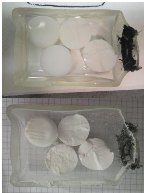
Figure 2-34: Picture of gels before (top) and after (bottom) SCD
