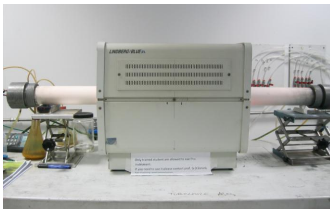
Figure 2-5: High temperature tubular furnace Lindbergh Blue
