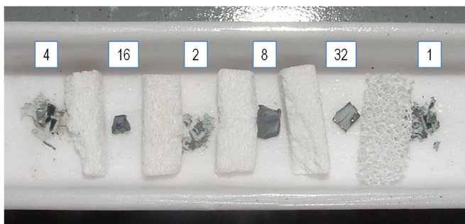
Figure 3-20: Appearance of the ceramic aerogels after the oxidation treatment
