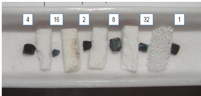
Figure 3-19 : Appearance of the ceramic aerogels before the oxidation treatment
