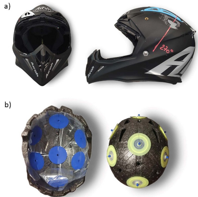
Figure 6. (a) Front and lateral views of Airoh Aviator 2.3 helmet. (b) EPS liners of the helmets with pads and sliding layer before the final assembly.
