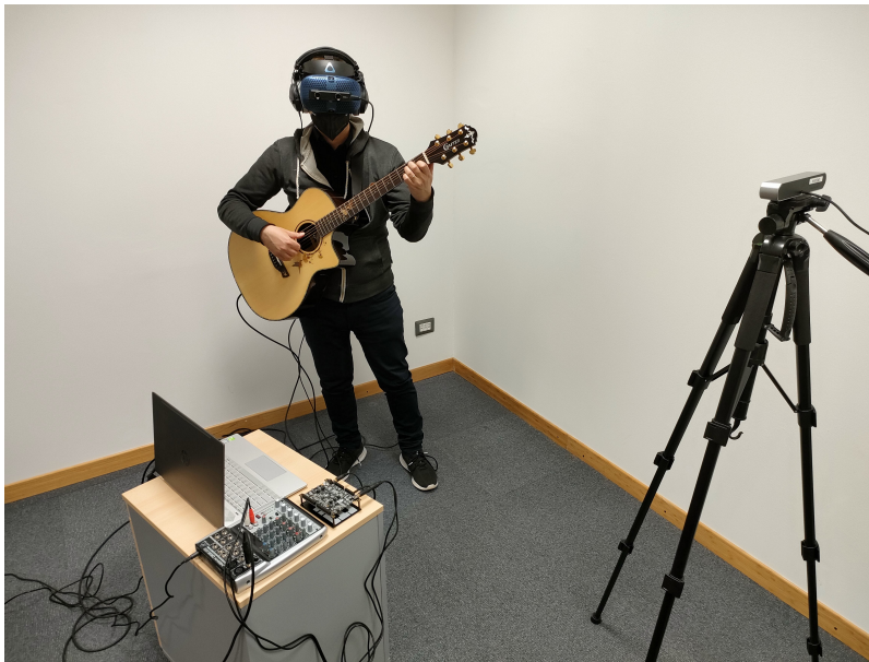
Figure 1: A picture taken during the testing phases of the proposed networked musical XR solution. The participant, while playing the instrument is able to visualize the virtual scene with the other musicians. As it can be seen the whole architecture consists of off-the-shelf hardware, that can be easily configured to suit the application scenario.
