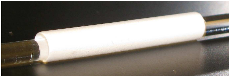
Figure 2-7. PCL tubular construct prepared by electrospinning.
