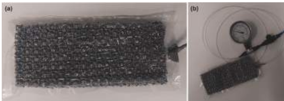
Fig. 2. Beam-like in-vacuo composite structure formed by a core strip structured fabric coated in an airtight plastic bag (a), which is deflated via a small suction pipe (b).
