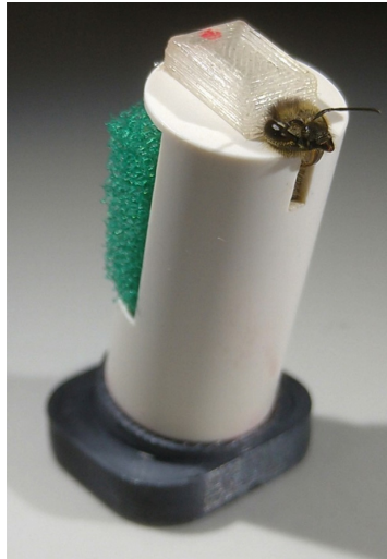
Figure 3.7.: Picture of bee in the bee holder, showing the head holder at the top and the sponge at the back
