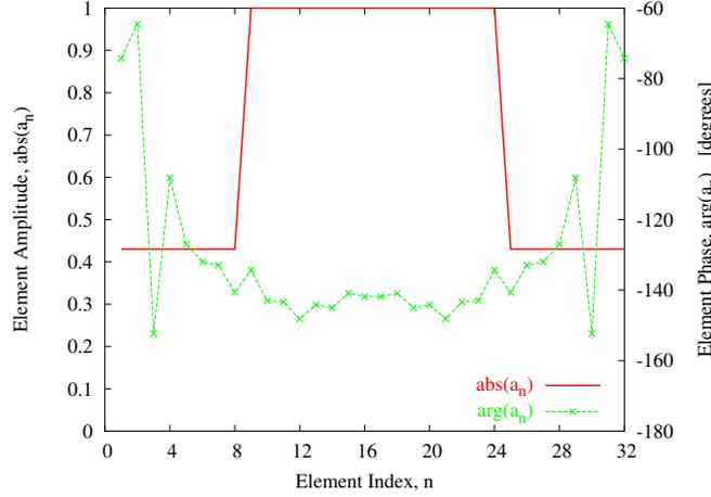
Fig. 5. Experiment 2 ( $N = 32$ ,  $Q = 2$ ) - Plots of the amplitude and phase values of the element excitations.
