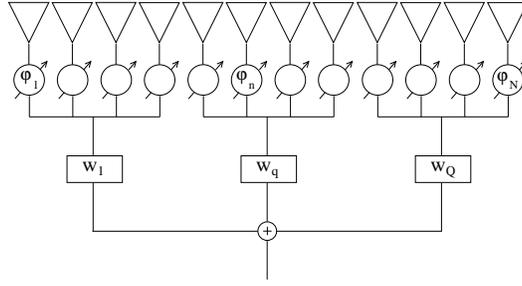
Fig. 1. *Array Architecture Geometry* - Example of a uniform sub-arrayed linear array antenna.
