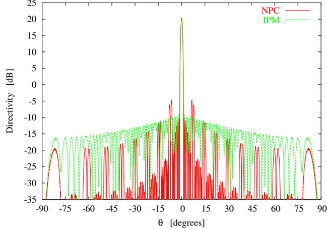
Fig. 2. Experiment 1 ( $N = 128$ ,  $Q = 4$ ) - Beam patterns synthesized with (IPM) and without phase control (NPC).
