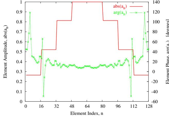
Fig. 3. Experiment 1 ( $N = 128$ ,  $Q = 4$ ) - Plots of the amplitude and phase values of the element excitations.
