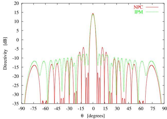
Fig. 6. Experiment 2 ( $N = 32$ ,  $Q = 2$ ) - Beam patterns synthesized with (*IPM*) and without phase control (*NPC*).
