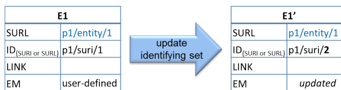
Figure 9.3: Updating an existing identifying set of an entity with SURI .
