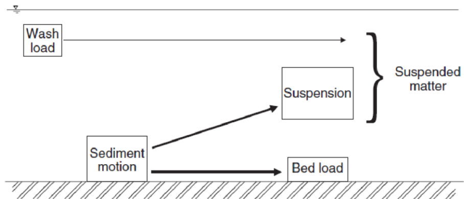
Figure 4. 11. Conceptual diagram of the different modes of sediment transport in rivers (Chanson, 2004)
