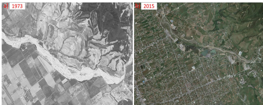
Figure 1. 6. Terkuze River (Ishem river basin) near Tirana Airport. (a) Corona images 1973 (reach 5) and (b) satellite image of 2015, showing urbanization and buildings very close to the river channel, which at the same time has been dramatically narrowed.
