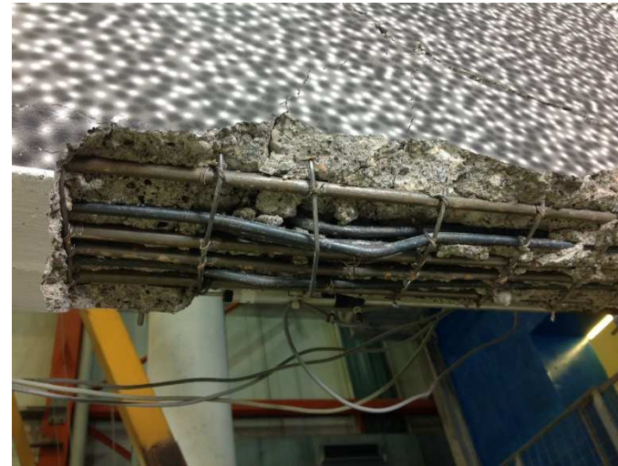
Column ends uplifting, expulsion of concrete covers
