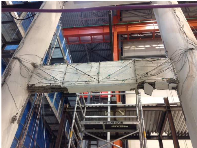
Column ends uplifting, expulsion of concrete covers
