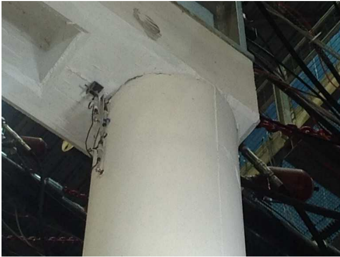
Column ends uplifting, expulsion of concrete covers
