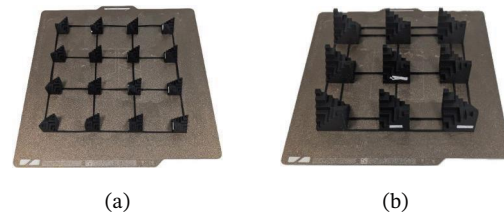
FIGURE 3 | FDM-printed modified COMPAQT staircase parts on the build plate: (a) 18 \times 18 \times 18 mm 3 arranged in a 4 \times 4 grid layout, and (b) 36 \times 36 \times 36 mm 3 arranged in a 3 \times 3 grid layout.
