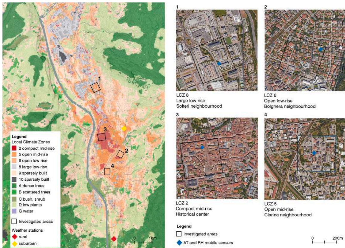
Fig. 2. LCZs classification of Trento, Italy, investigated areas and location of the weather stations.
