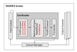
Figure 7.7: PADRES router extended with encryption functionality.
