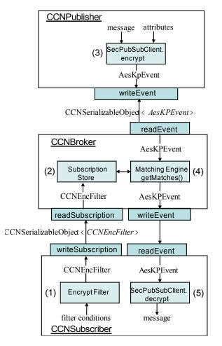
Figure 7.5: Encrypted routing over CCNx.
