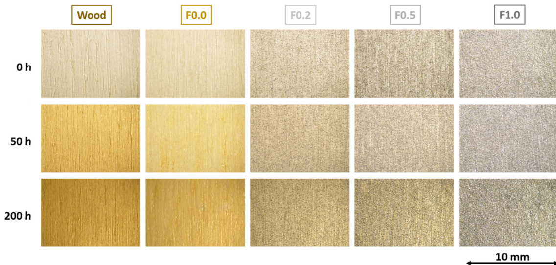
Fig. 6: Change of the appearance of the coated samples and the wooden reference panel during the exposure to UV-B radiation
