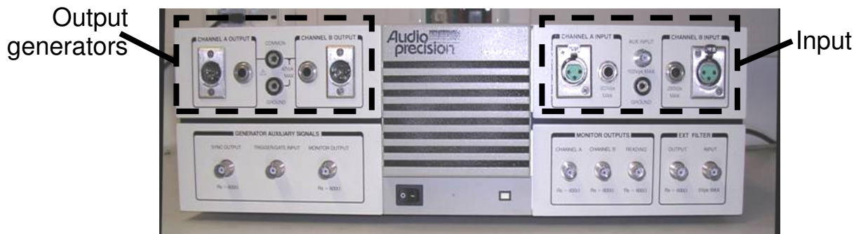
Figure 4.21 Audio analyzer Audio Precision System One. Acquire data from DUTs and it can generate signals
