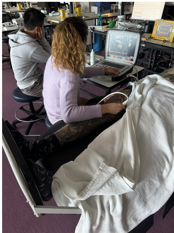
Figure D.7: Experimental setup. Duplex Doppler ultrasound of the femoral artery of a volunteer positioned at 60^\circ .
