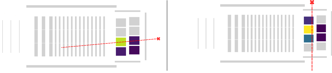
Figure 4.2: Representative event-display views of simulated gamma-ray interactions in CALOG for the horizontal (left) and vertical (right) acceptance windows. The dashed red line indicates the reconstructed photon trajectory; colored crystals mark energy deposition in the CALOG matrix.
