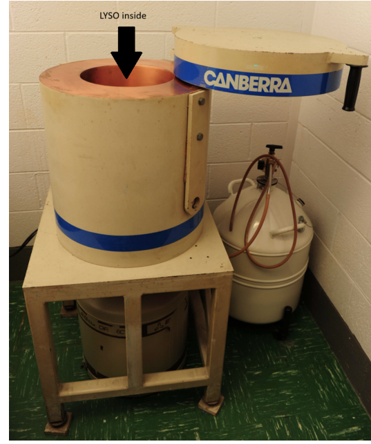
Figure 2.5: (a) Schematic cross section of a typical HPGe detector cryostat, illustrating the liquid-nitrogen dewar, cold finger, and the vacuum-sealed germanium crystal mounted behind the detector endcap. Adapted from Khater [88], (b) The HPGe detector and internal copper lining installed inside a lead shielding assembly. The upper shielding chamber accommodates the sample placement region in front of the detector end, while the cryostat and liquid-nitrogen dewar are located below the shielding structure. 2
