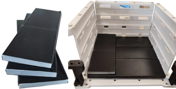
Figure 3.7: Photograph of PST structural model realized during the integration phase. In the flight model, aluminum foil replaces the black vinyl tape used during prototyping (Image courtesy of the NUSES Collaboration).
