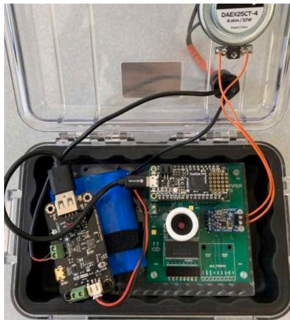
Fig. 20. Shows added solar charge controller.
