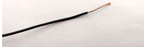
Fig. 10. Exposed end of the contact microphone wire after removing the connector and stripping off 2 cm of insulation.
