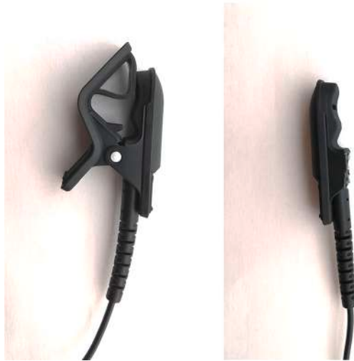
Fig. 11. Before and after removing the mounting clip from the contact microphone.
