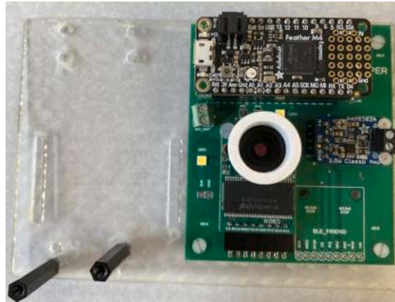
Fig. 17. Case with gland installed in hole.
