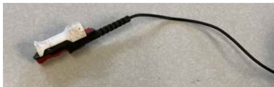
Fig. 14. contact microphone completed with 3D printed attachment.
