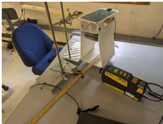
Fig. 21. Experimental apparatus used to measure the frequency response of the audio output system. The trap and artificial substrate (meter stick) are suspended using laboratory stands in a manner consistent with the trap’s field mounting conditions.
