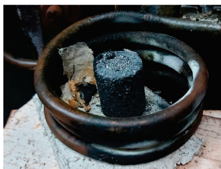
Figure 1. Melting the charge in the graphite crucible.
