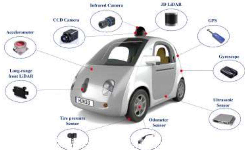
Figure 4. Main sensors used in CAVs.
