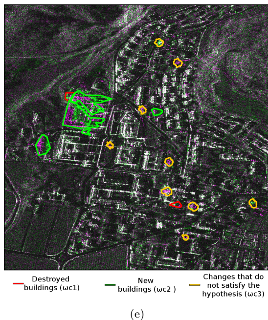
Figure 3.12: Trento (Italy) data set: (a) optical image (2011 [85]); and (b) RGB multitemporal composition of spotlight TerraSAR-X and TanDEM-X images (R:03/04/2013, G:21/01/2011, B:03/04/2013). (c) Change detection map \mathbf{M}^{\text{opt}} obtained at the level N - 1 = 3 . (d) Map showing the index of the size of changes \mathbf{C} . (e) Changed building map overlapped to the RGB multitemporal composition of CSK data.
