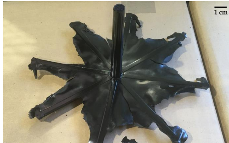
Figure 1. Example of injection moulding sprue used as recycle in the mechanical recycling process.
