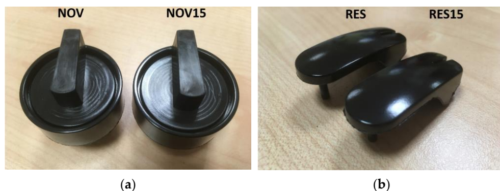
Figure 10. Representative images of knobs produced upon industrial production trials based on (a) NOV and NOV15 samples, and (b) RES and RES15 samples.
