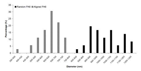
Figure 4.8: Histogram representing the random and aligned PA6 fiber diameter distribution.
