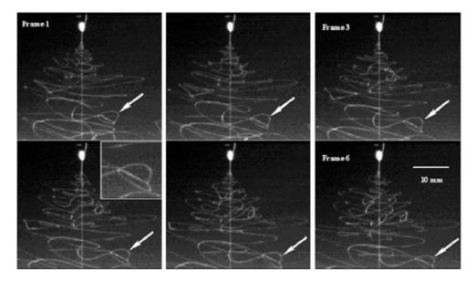
Figure 2.9: Trajectories of the jet in the whipping instability region during the electrospinning of PCL in 15 wt% acetone solution (applied voltage is 5 kV and gap distance is 14 cm). [5]
