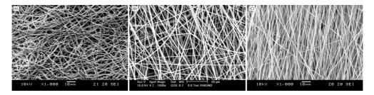
Figure 4.5: The influence of applied voltage on the fiber alignment of PA6, when the target tangential speed is 3.33 m/s. (A) 20 kV, (B) 15 kV and (C) 5 kV.
