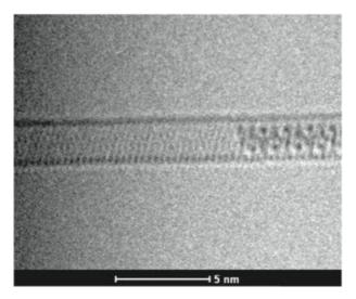
Figure 2.3: TEM image of a single-walled carbon nanotube. (http://www.electroiq.com).
