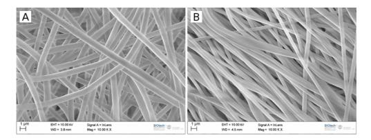
Figure 4.6: Random PA6 (A) and aligned PA6 (B) produced networks.
