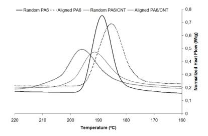
Figure 4.15: Partial thermogram depicting the crystallization region.
