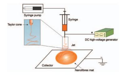
Figure 2.7: Most common electrospinning apparatus. [3]
