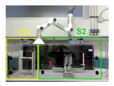
Figure 3.3: Electrospinning safety box, S1 shows the static system and S2 the dynamic system.
