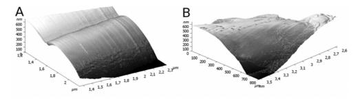
Figure 4.11: AFM images depicting the surface topography of the (A) PA6 and (B) PA6/CNT fibers.
