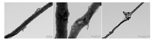
Figure 4.10: Transmission electron micrography of PA6/CNT electrospun fiber.
