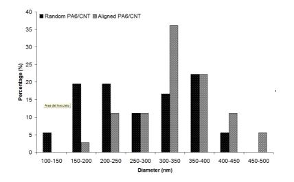
Figure 4.9: Histogram representing the random and aligned PA6/CNT fiber diameter distribution.
