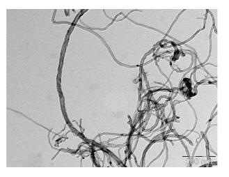
Figure 4.1: TEM image of the supplied multi-walled carbon nanotubes.
