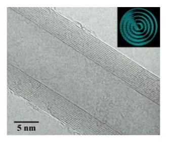
Figure 2.4: TEM image of a multi-walled carbon nanotube. (http://endomoribu.shinshu-u.ac.jp/).
