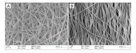
Figure 4.7: Random PA6/CNT (A) and aligned PA6/CNT (B) produced networks.
