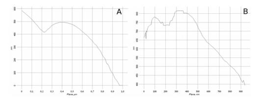
Figure 4.12: Fiber profile acquired from the AFM images, (A) PA6 and (B) PA6/CNT.
