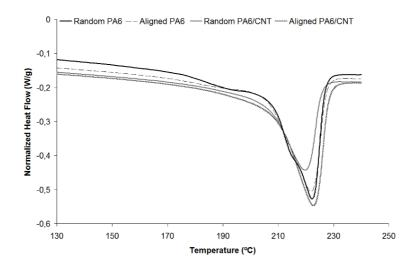
Figure 4.16: Second scan partial thermogram depicting the melting region.
