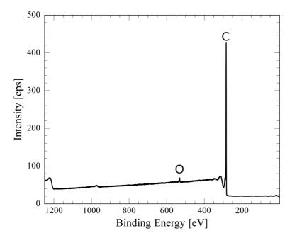
Figure 4.2: XPS survey spectra of the supplied MWCNTs.
