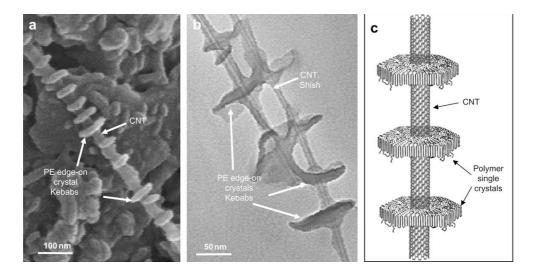
Figure 4.17: PE/MWCNT NHSK structure produced by solution crystallization of PE on MWCNTs at 103 °C in p-xylene for 30 min. (a) SEM image of MWCNTs decorated by disc-shaped PE single crystals. (b) TEM image of the PE/MWCNT NHSK structure. (c) Schematic representation of the PE/CNT NHSK structure. PE forms lamellar single crystals on CNT surface with polymer chains parallel to the CNT axis. [6]
