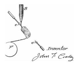
Figure 2.5: Electrospinning diagram drawn by Cooley in 1902, where A is a solution of polymer (e.g., collodion or cellulose nitrate in ether or acetone) delivered into the high-voltage direct current (DC) electric field via tube B to form electrospun nanofibers collected on a drum F. [1]
