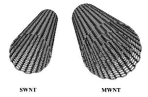
Figure 2.2: Molecular structures of a single-walled carbon nanotube (SWCNT) and of a multi-walled carbon nanotube (MWCNT). (http://www-ibmc.u-strasbg.fr/).
