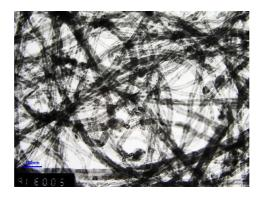
Figure 3.2: TEM micrography of the supplied MWCNTs. Source: Cheap Tubes.
