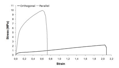
Figure 4.18: Typical stress-strain curves of orthogonal and parallel regarding the spinning direction.
