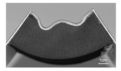
Figure 6.6: Bifurcation of a two-layer rubber block under finite bending evidencing long-wavelength bifurcation modes. Stiffness and thickness ratios between the layers are  $(2.687 \text{ N/mm}^2)/(0.095 \text{ N/mm}^2)$  and (3 mm)/(40 mm), respectively. The stiff layer (86 mm × 3 mm × 150 mm, made up of natural rubber, marked with a white pencil on the sample) is at the compressive side and coats a neoprene layer (86 mm × 40 mm × 150 mm).
