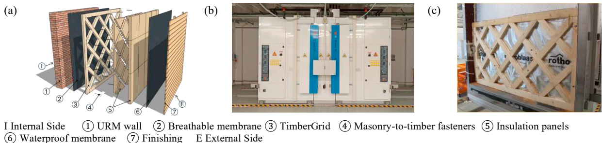
Fig. 10. Energy efficiency assessment: (a) insulating layers; (b) climatic chamber; (c) external side of wall specimen with breathable membrane and timber grid
