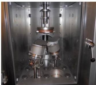
Figure 37: Sputtering system Oerlikon Leybold Univex 450B.
