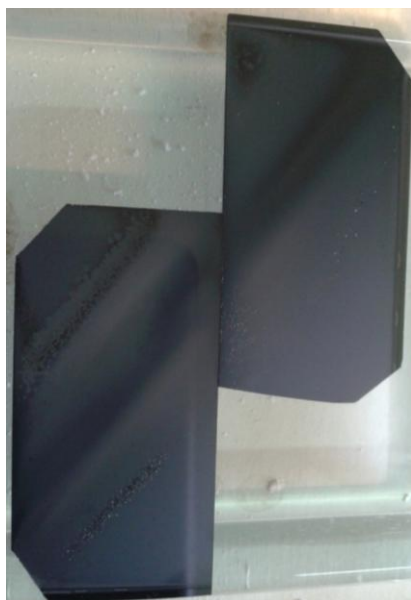
Figure 95: Picture of two portions of a sulphurized sample containing the [\text{Cu}]/[\text{Sn}] \approx 2 stripe
