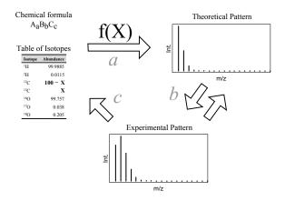
FIGURE 4.4: Exemplified scheme showing how *IsotopicLabelling* works. In this example, a  $^{13}$ C-based experiment is considered.
