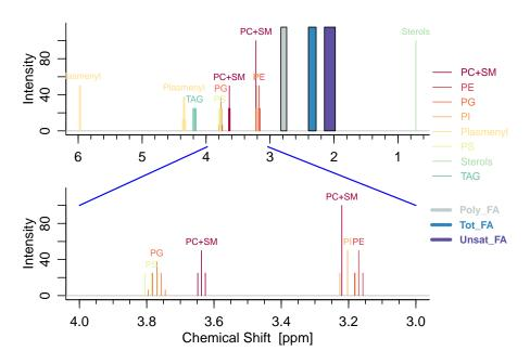
FIGURE A.1: Synthetic NMR spectrum showing characteristic resonances of the most common lipid classes, with a zoom in of the crowded 2–3 ppm chemical shift region. Many are the signal overlaps, making it difficult to unequivo-cally assign the resonances.
