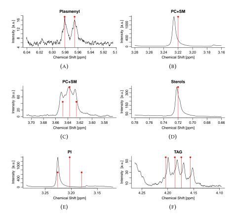
FIGURE A.5: Examples of the graphical outputs produced. The experimental spectrum is dissected and the characteristic regions are plotted together with the theoretical resonances (red vertical lines); it is up to the researcher to understand whether or not the considered class is present.
