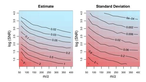
FIGURE 4.13: *Left:* minimum <sup>2</sup>H percentage abundance (black level curves) for which the difference between labelled and control patterns is significant. *Right:* related standard deviation. The sensitivity strongly depends on the analyte size and on the SNR.
