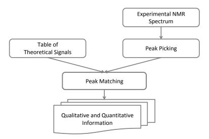
FIGURE A.4: Block diagram of the informatics tool aimed at helping in the interpretation of NMR spectra of lipid mixtures.
