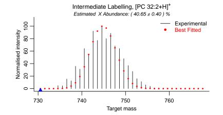
FIGURE 4.9: Example of extracted pattern for [PC 32:2+H]<sup>+</sup>, intermediate labelling. The pattern shows a peculiar saw-tooth shape that is not accounted for by our isotopic pattern analysis.
