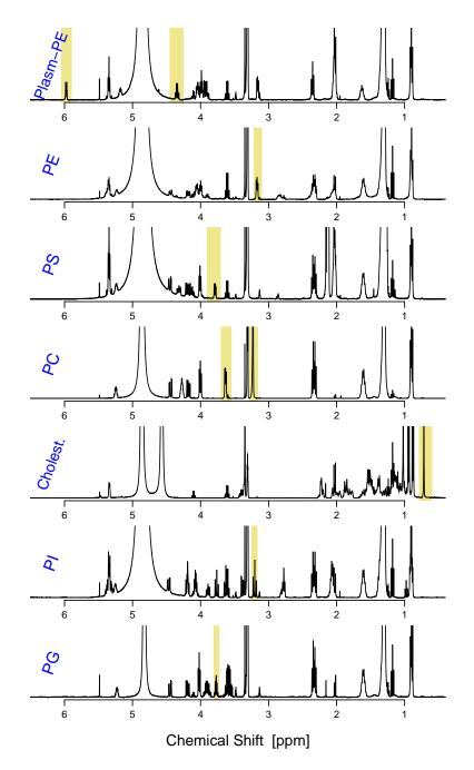
FIGURE A.2: Experimental NMR spectra of the most common lipid classes. Yellow rectangles highlight the characteristic resonances of each class.
