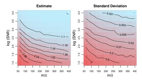
FIGURE 4.12: *Left:* minimum <sup>13</sup>C percentage abundance (black level curves) for which the difference between labelled and control patterns is significant. *Right:* related standard deviation. The sensitivity strongly depends on the analyte size and on the SNR.
