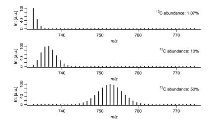
FIGURE 4.3: Simulated MS isotopic patterns for [PC 32:1+H]<sup>+</sup>, assuming different <sup>13</sup>C abundances. The underlying assumption here is that the label is uniformly distributed over the C sites of the considered molecule, with the specified average abundance.
