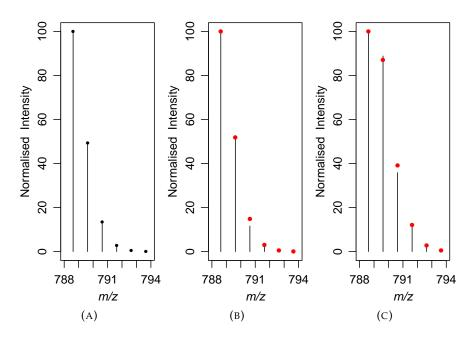
FIGURE 4.15: Comparison between the isotopic patterns of [PC 36:1+H]<sup>+</sup>: (A) natural pattern, (B) experimental pattern of one of the least enriched samples, and (C) experimental pattern of one of the most enriched samples. The red dots are the best-fitted patterns.
