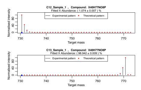
FIGURE 4.6: Two of the extracted patterns for [PC 32:2+H]<sup>+</sup>, with their best-fitted patterns (red dots). The estimated <sup>13</sup>C abundances are given with the SER.
