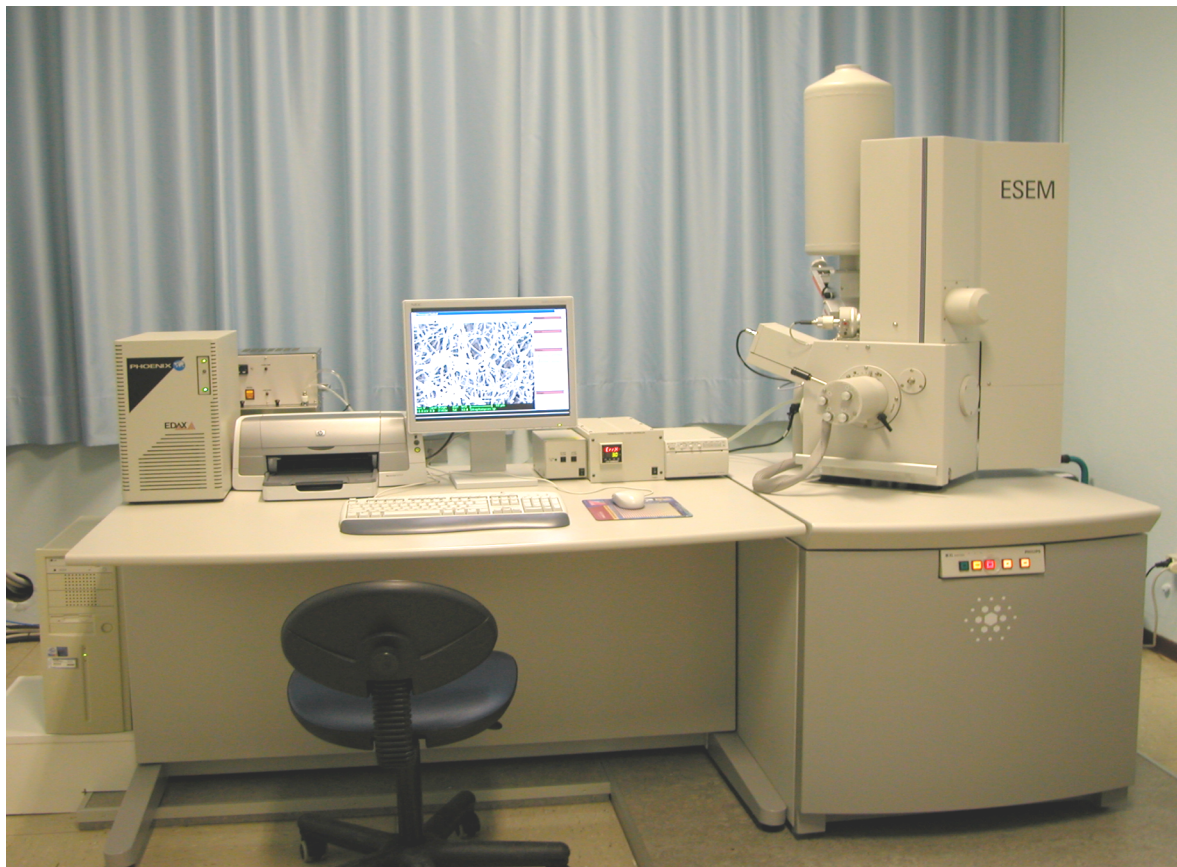
Figure 8. Scanning Electron Microscope (SEM) FEI XL 30 ESEM FEG in the Department of Medicine Laboratory, APSS, Trento.
