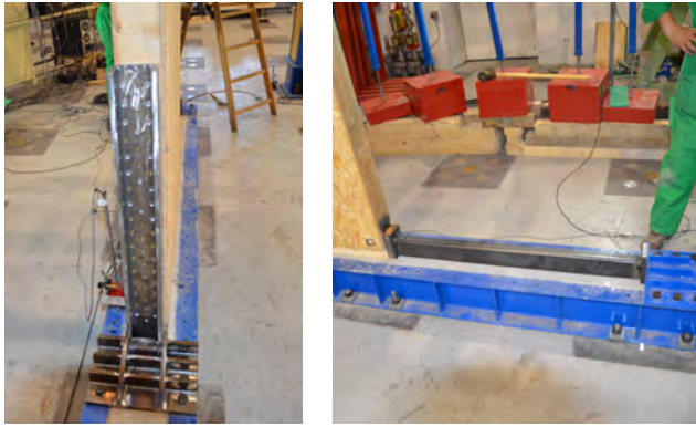
Figure 20: Connecting-devices: hold-down and locking rectangular tube
