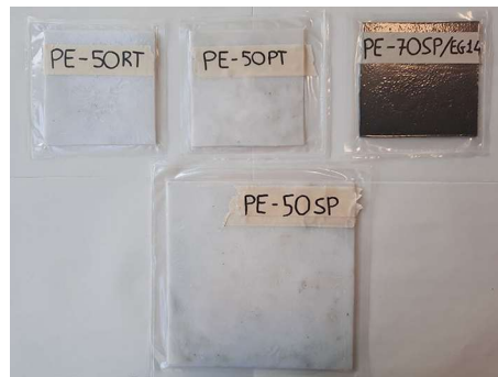
Figure 8. PE enveloped panels having dimensions 120 × 120 × 3 mm 3 (top) and 200 × 200 × 3 mm 3 (bottom).
