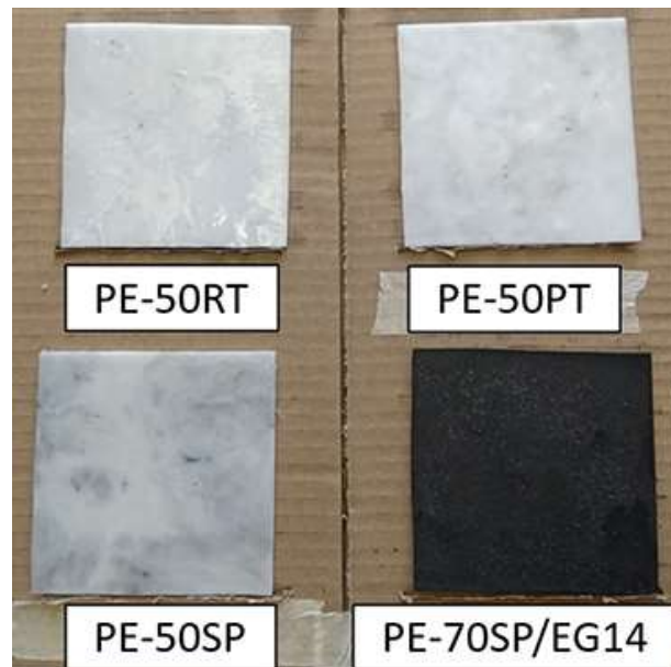
Figure 1. Sheets of PCM-HDPE composites ( 120 \times 120 \times 3 \text{ mm}^3 ) placed on a paperboard and observed with IR thermography.
