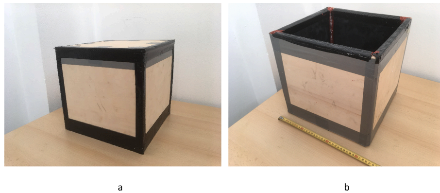
Fig. 1. Representative picture of the boxes (volume = 0.27 m 3 ) used for the tests: top view (a) and bottom view with E-PCM insulation (b).
