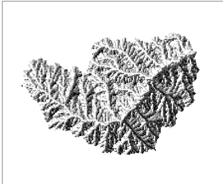
Figure 4.2: Example of drainage direction map for the Little Washita basin, OK, USA.
