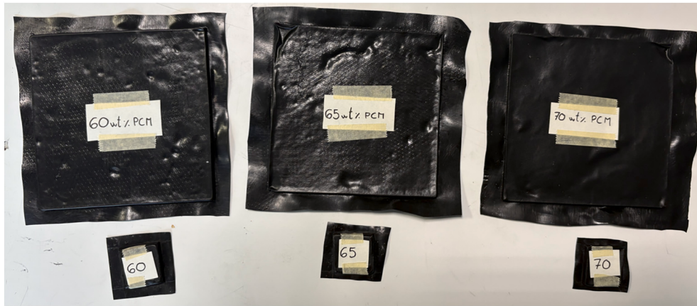
Fig. 2. Representative image of EPDM-60RT28/12EG, EPDM-65RT28/12EG and EPDM-70RT28/12EG samples (left to right). Top: 120 mm × 120 mm × 5 mm panels. Bottom: 25 mm × 25 mm × 5 mm panels.
