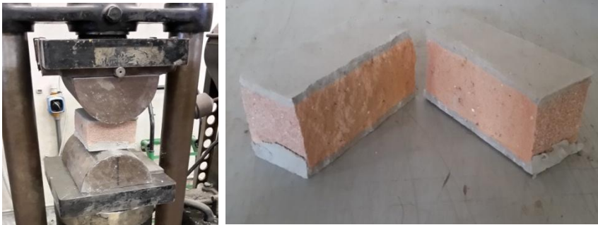
Fig. 5.19 Splitting test, the testing machine (left) and the brick failure (right)
