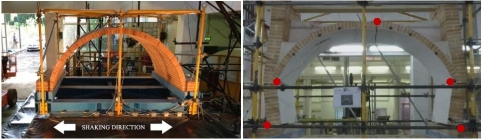
Fig. 2.71 Shaking table tests in the framework of ProVaCI research project
