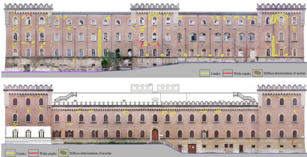
Fig. 4.7 Crack pattern and damage survey of the North (above) and South (below) façade.
