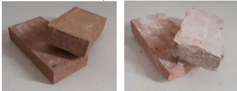
Fig. 5.17 Specimens of new bricks (NB) (left), and historical bricks (HB) (right)
