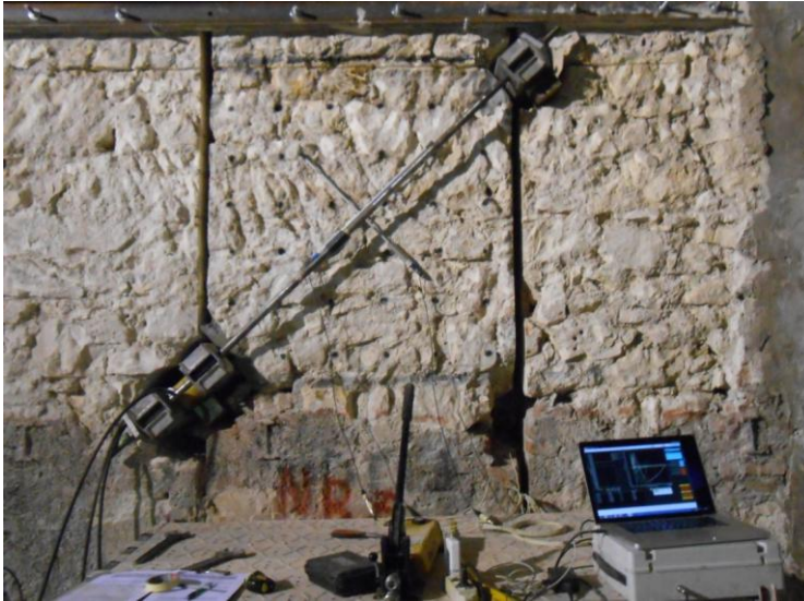
Fig. 3.1 Diagonal compression test of one specimens, the black dots refers to the sonic grid
