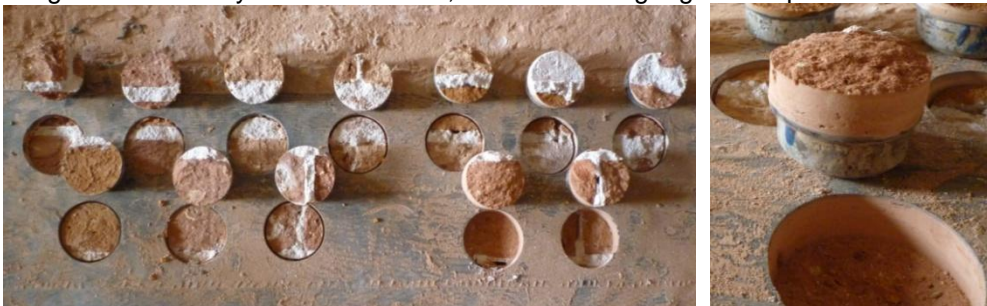
Fig. 5.27 Pull-off failures of CFRP
