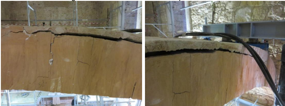
Fig. 5.60 Compressive failure of masonry between the keystone and the loading point
