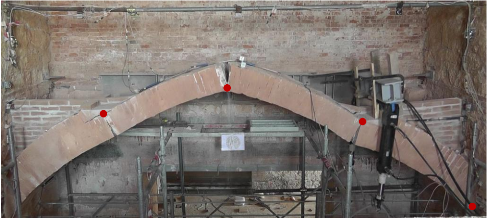
Fig. 5.40 Vault with diaphragms prior to collapse
