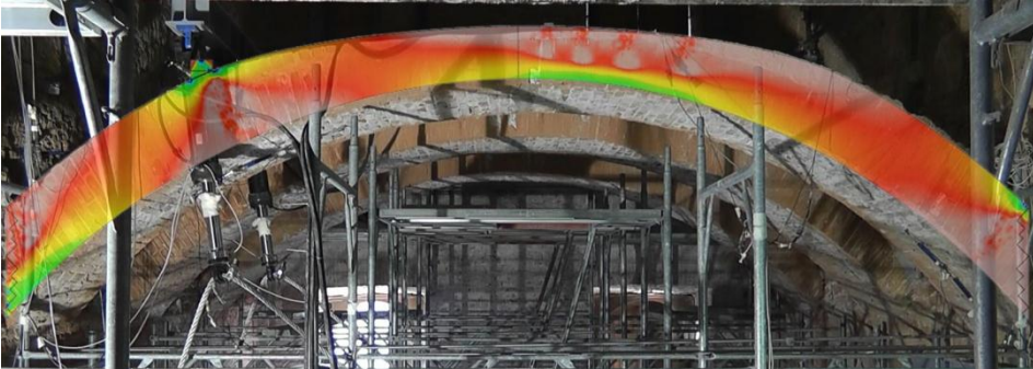
Fig. 6.71 Principal compressive stress plotted on SRG vault
