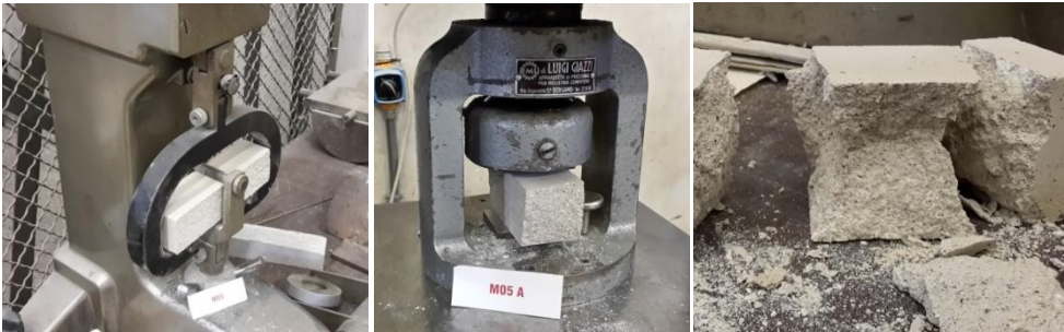
Fig. 5.24 Flexural testing of mortar prism (left), compressive test (centre) typical failure (right)
