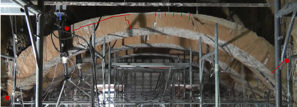
Fig. 5.55 SRG vault after the reaching of the maximum displacement
