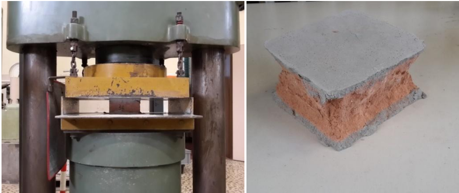
Fig. 5.22 Compressive test, the testing machine (left) and the typical brick failure (right)
