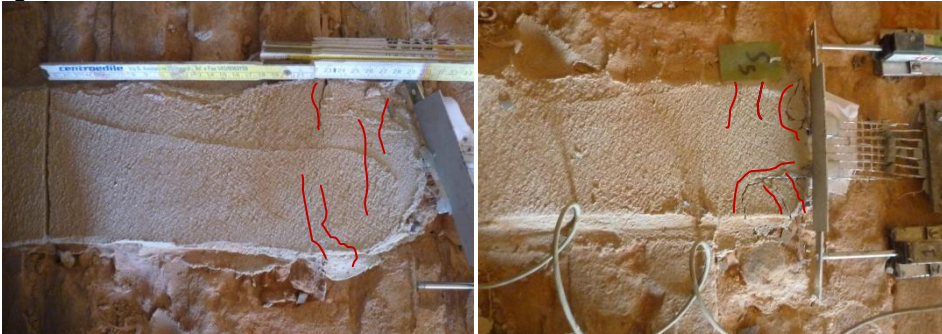
Fig. 5.31 Cracks spreading in shear test on two specimens
