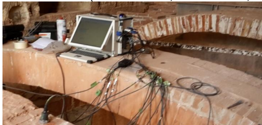
Fig. 5.80 Acquisition system (NI PXI-1042Q) and accelerometer (PCB 393 B12)
