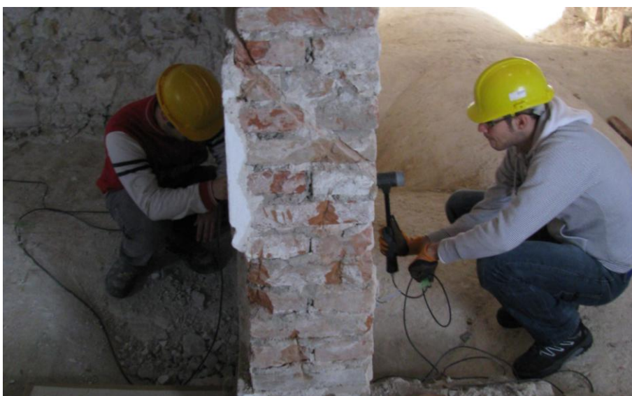
Fig. 2.20 Direct sonic test execution, instrumented hammer (left) and accelerometer (right)
