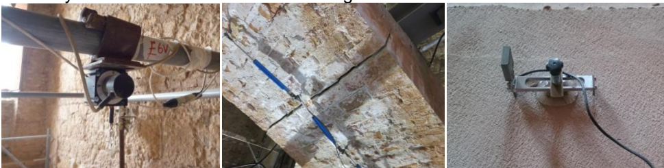
Fig. 5.5 Wire trans. (left), linear displacement trans. (centre), strain sensor (right)
