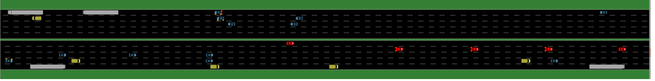
Figure 3. Screenshot of the realistic scenario showing the platoon (red cars) performing the join at the tails maneuver.
