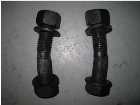
Figure 5.44 - Experimental and numerical specimen deformations for \varphi = 45^\circ
