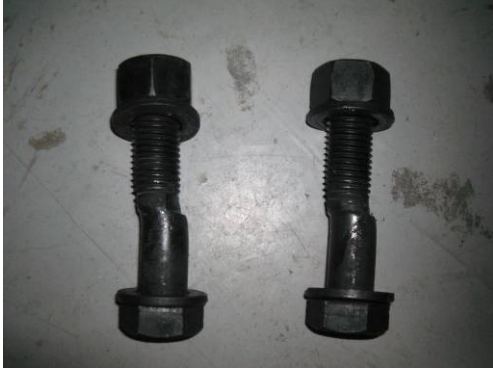
Figure 5.43 - Experimental and numerical specimen deformations for \varphi = 15^\circ
