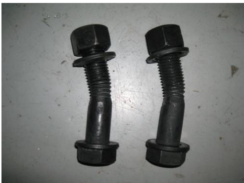
Figure 5.45 - Experimental and numerical specimen deformations for \varphi = 75^\circ
