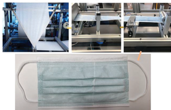
Figure 4. Overview of the process to rotary-print three-layered medical face masks with TMB. The top left image shows bulk textile-roller folding to make it ready for printing on one side of surface as in the middle image, and the right image shows shape formation of printed fleece folded into mask; bottom shows TMB-printed mask produced in industrial scale.
