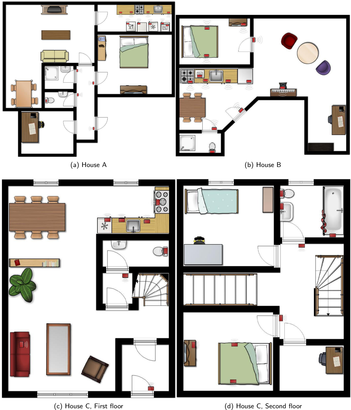
Figure 3.1: Floor plans of houses A, B, and C for van Kasteren Dataset. Sensors are depicted as red boxes (Taken from (van Kasteren et al., 2010b))
